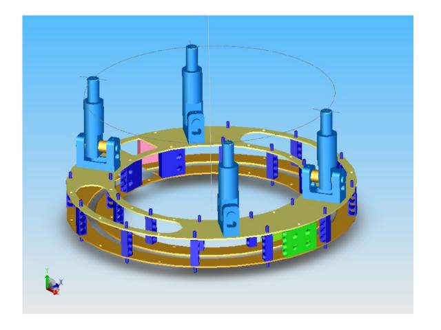
The oven encloses the circular sample track and is completely non-magnetic. Hot air is guided through copper pipes which heat the samples by radiation.
