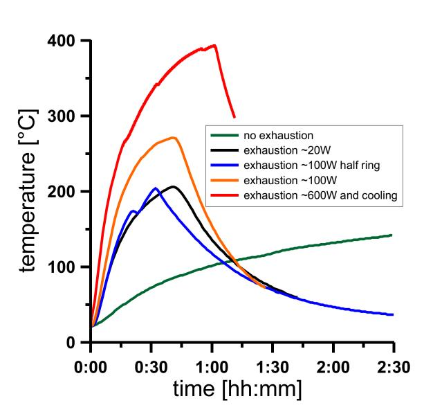
Initially, the new hot air heating concept was limited to temperatures up to 140°C (green). After improving the air circulation, 400°C can now be achieved (red).
