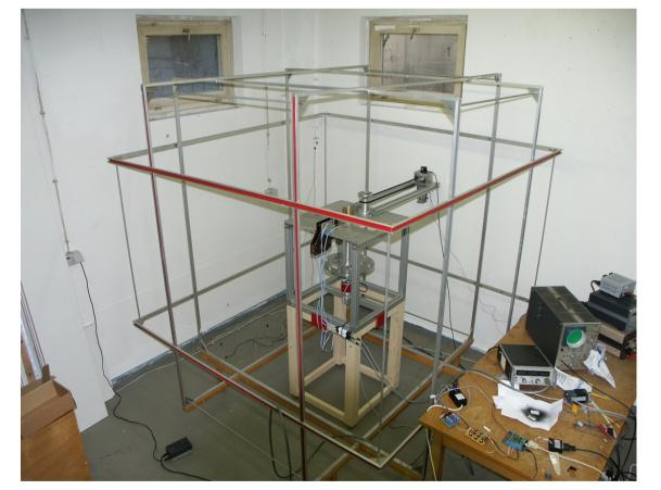
The Hotspin 2 spinner magnetometer is enclosed by three Helmholtz coils (photo on the left side) to generate a field free environment for the demagnetisation process. Main mechanical features are the rotating sample platform below the circular oven and the sensor holder (sketch on the right side).
