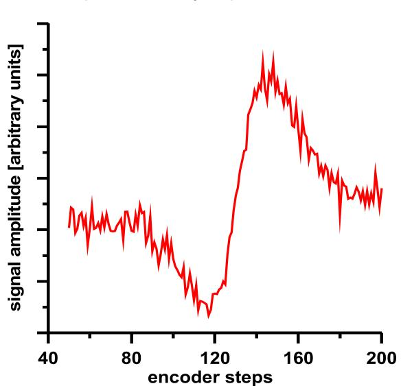
Magnetic signal (z-component) of sample AGA9\_2 with a magnetization of 55 mA/m measured by Hotspin 2. The noise level is in the order of 10 mA/m.
