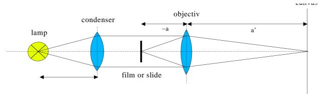
The lamp should be in the absolute focus of the condenser lens to get parallel beams on the other side. For a and a' the following equation applies:
