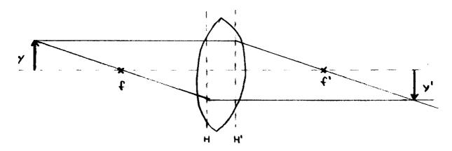
Exercise 3.3.4 Calculate the focal distance of the system's dispersion lenses from the focal distances determined in 3.3.1 and 3.3.2 by means of equation (6) with t = 40 mm
