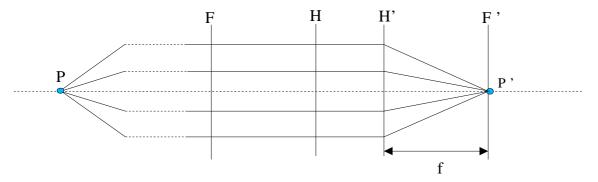
If you assume that P is indefinitely far away, all beams of light are parallel and focused in the focal layer in P'. So the distance between the main layer and the film should be the focal distance (200 mm), to get a sharp image.
